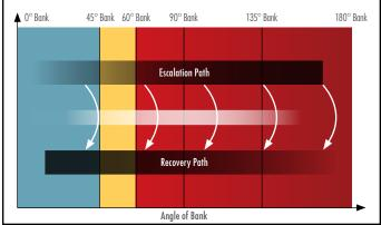
The intent of UPRT is to provide pilots with the ability to recover regardless of how severe the upset becomes. The pilot should be able to effectively apply a mitigation strategy to any flight condition, applying an appropriate remedy to return the aircraft to the desired attitude.
